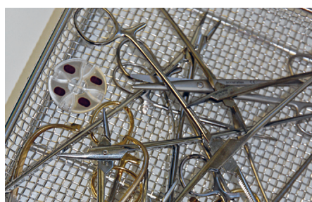
The sensors are designed to avoid flipping and illustrate the cleaning quality of the rinsing process.
