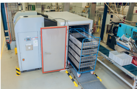
Conditioning means that the absorption of water in the plastic over several months is realised within a few hours.
