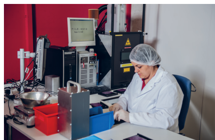
The caps are coded by laser to facilitate clear identification of samples in the lab.
