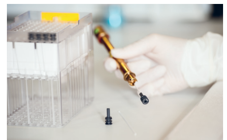
The glass tubes are fitted with the coded caps and then assembled in a rack with 96 sample tubes.
